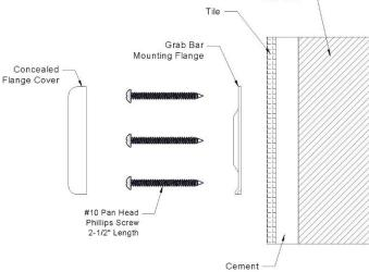
Apply a bead of silicone around the Grab Bar Mounting Flanges on the mounting surface to ensure a water-tight seal will be created at all mounting locations. Secure the grab bar to the wall using six (6) #10 x 2-1/2" stainless steel screws (supplied by manufacturer) and screw into the 3/32" holes created in the solid wood backing. *Tighten screws*
